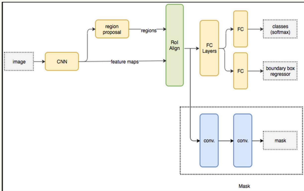
Figure 4 Mask R-CNN Architecture [7]
