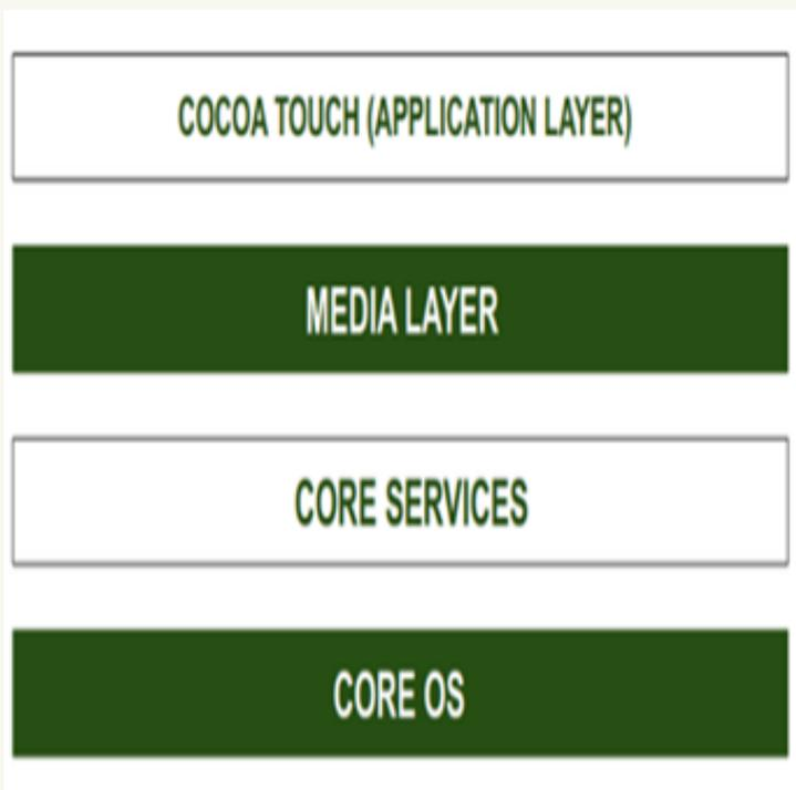
Figure 5: Architecture of the iOS Operating system [10]
